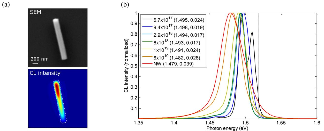
Figure 1: (a) SEM image and CL intensity map of a single Be-doped GaAs NW. (b) 20K CL spectra of GaAs films (p-doping levels are shown in  $\text{cm}^{-3}$ ) and of NW. (Peak energy, FWHM) of each spectrum are noted in eV. The vertical line indicates the GaAs bandgap.
