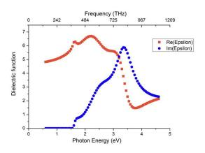
Dielectric function of cubic MAPbI obtained by ellipsometry
