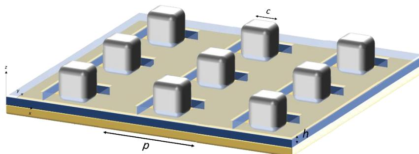
Fig1. Design of the rectenna nanocube-based array
