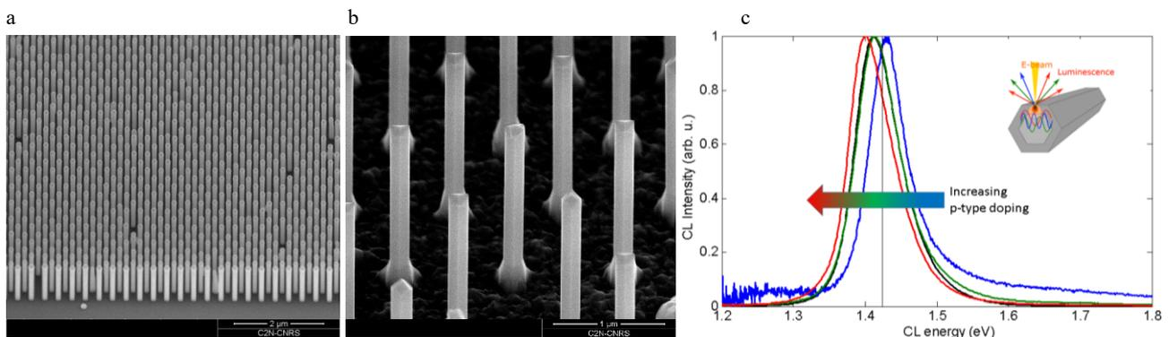
Figure (a): 45° SEM view of an array of GaAsP nanowires on Si (111), with catalyst still present at the end of the axial growth.
